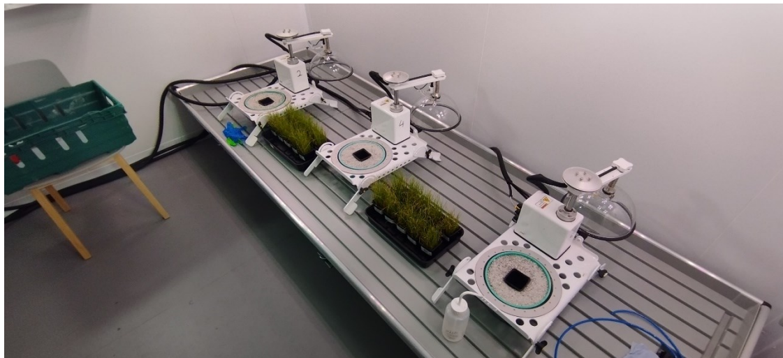
Figure 3. Automated gas measurement chambers formed by a transparent dome and an adapted ring for the pots used in this experiment.
