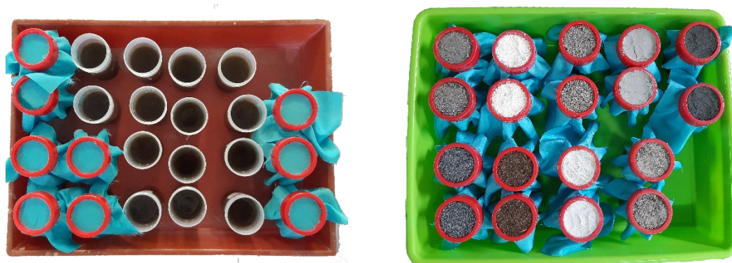
Figure 1. The experimental units used to test the filter combinations for capturing GHGs and \text{NH}_3 emissions.
