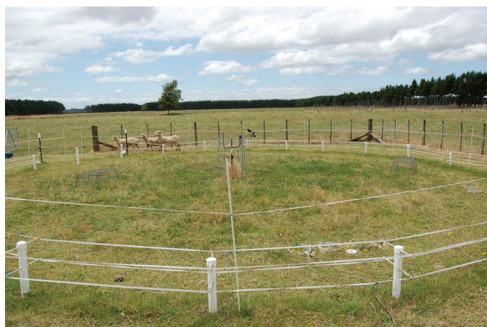
Plate 5. One of the rings that make up the FACE facility at Palmerston North. CO 2 concentrations are kept constant by emissions of CO 2 from stakes
